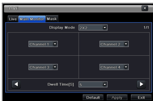
Fig 5-7 Live Configuration-Main Monitor
